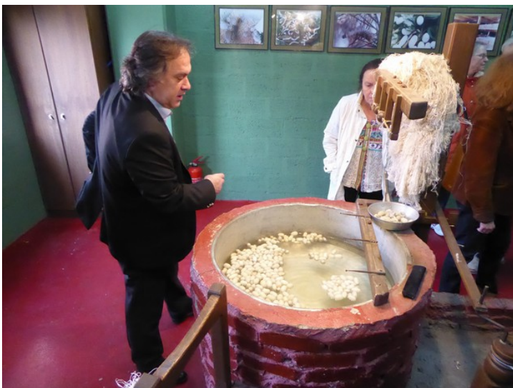
In the same room they wind up silk from cocoons located in a water bath.
