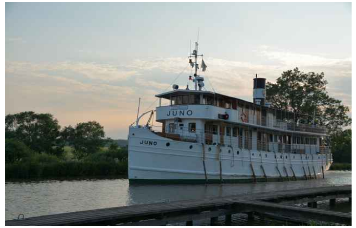
The fenders is hanging alongside to protect the hull when in the locks.
