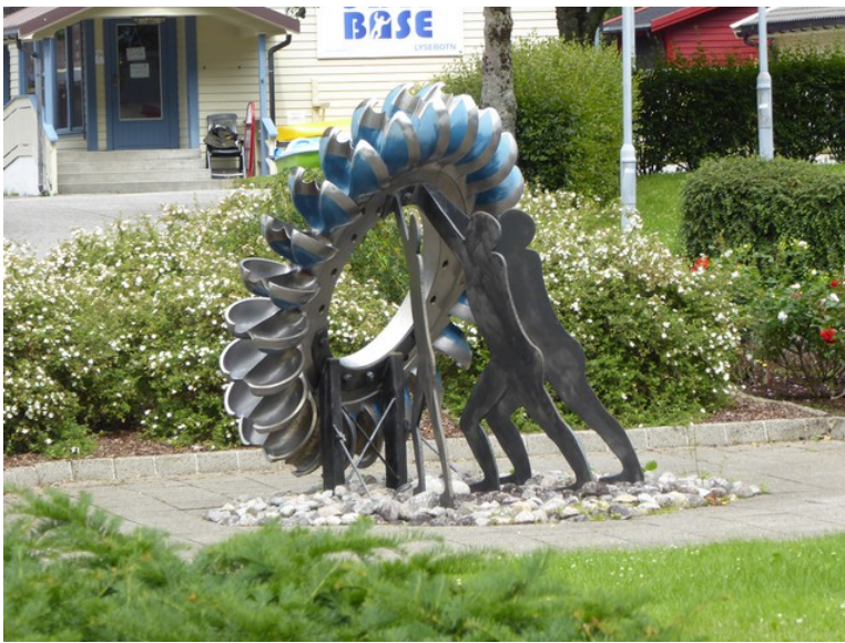
This is a paddle wheel that has been in a Pelton turbine .
