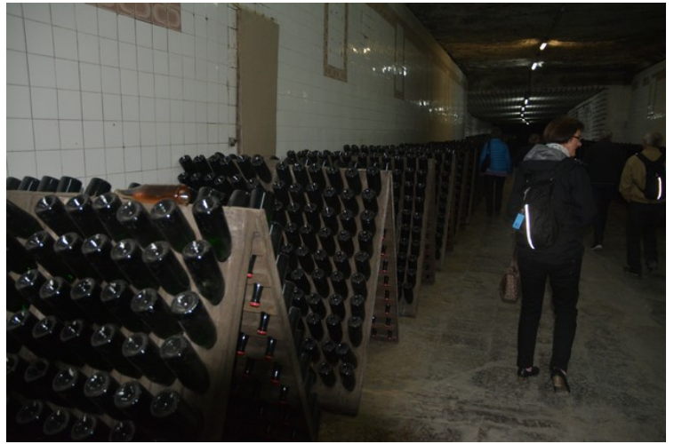
All these bottles must be rotated on a regular basis to secure the precipitate on the cork.
