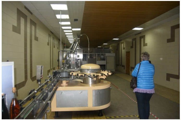
Machinery for tapping and corking sparkling wine.
