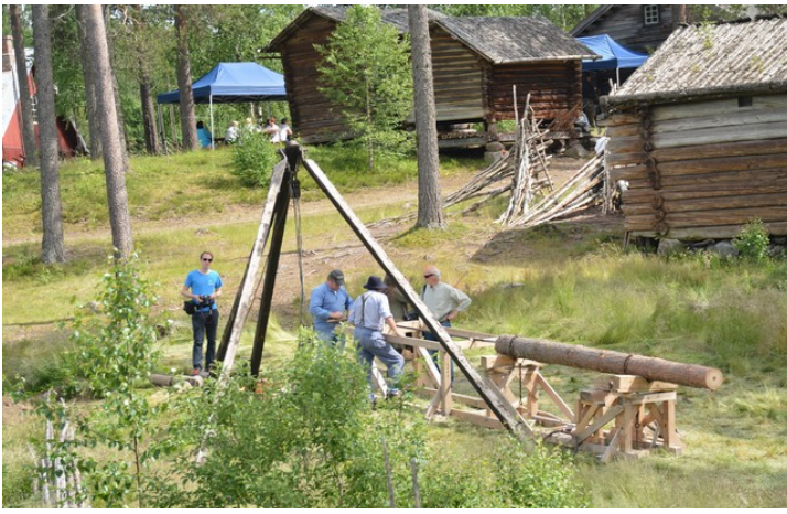
“Steinbukk” to lift stones and tree trunks out of the ground.
