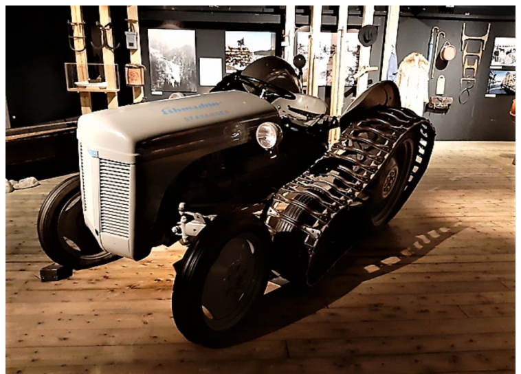
A Little Gray Fergie (Ferguson TE20) with belts was used in the forest.
